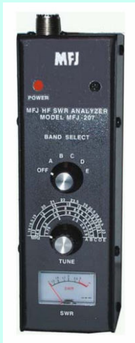
Example of a basic SWR Analyzer: MFJ 207
