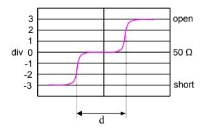
$Vf = 2.033 \cdot \frac{d}{t}$  Vf = velocity factor d = distance in feet t = tdr waveform delay in nS
