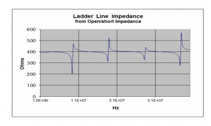
Example of Zo magnitude measurement on a ladder line. A 4:1 balun was used to improve the accuracy of impedance measurements (derived from S11). The peaks occur at line lenghts which are multiples of 90 degrees. These errors are caused by inaccuracies in measuring extreme values of impedance.
