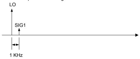
Move the LO up by 11 KHz, when the two tones are transmitted. The audio output will now give TWO tones at 10 and 15 KHz respectively. Record these in a .wav file for processing with SL, using a sampling rate above 30 KHz.
