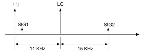
The LO should be moved from 30 to 40% of the expected span.
