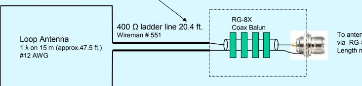
To antenna tuner via RG-8 / 11 Length not critical.
