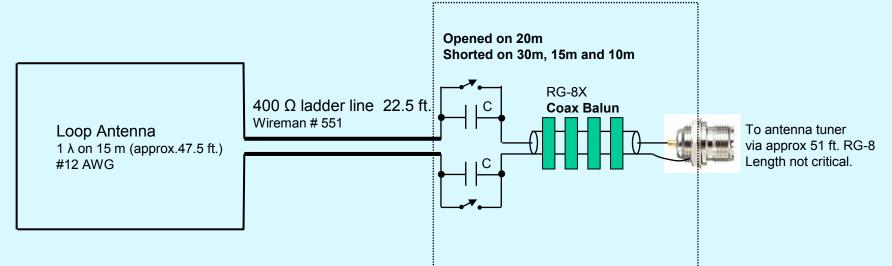
The length of the ladder line is approx.  $\lambda/2$  at 21 MHz. **Obtained from simulations.** The 90  $\Omega$  loop impedance is transformed to about the same value on 21 MHz.
